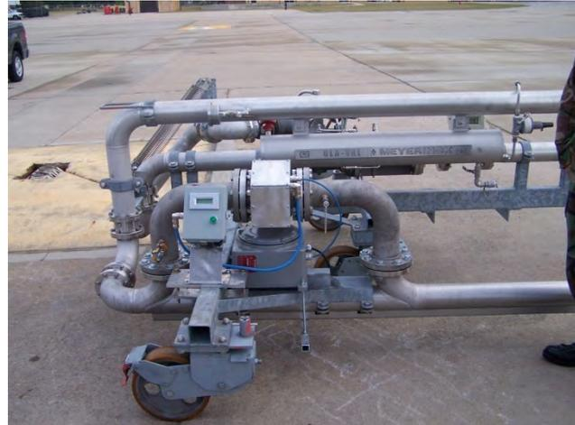
**PANTOGRAPH with Water/Solid Sensor**
