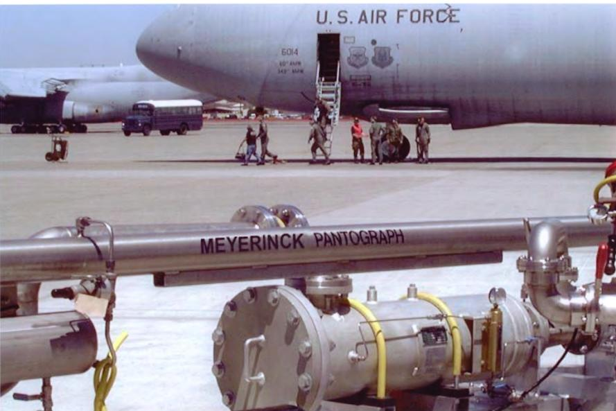
**PANTOGRAPH with Fuel Monitor**
