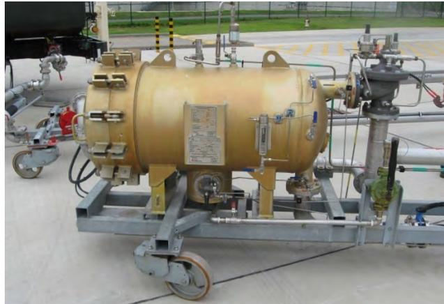
**PANTOGRAPH with Filter/Water Separator**
