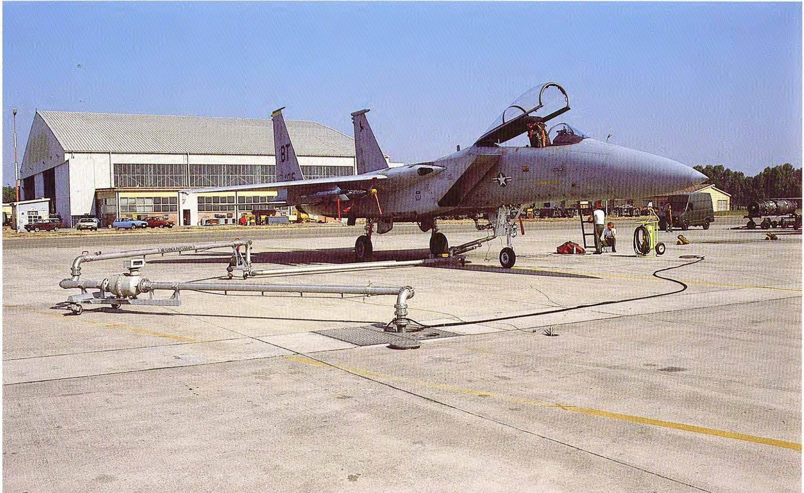
**CLA-VAL-Hot refueling PANTOGRAPH with flow meter and CLA-VAL hydrant pit valve**
